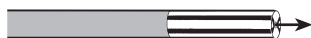
Fig. 5.29 The tip of a multipolar BICAP probe with a central water jet.
